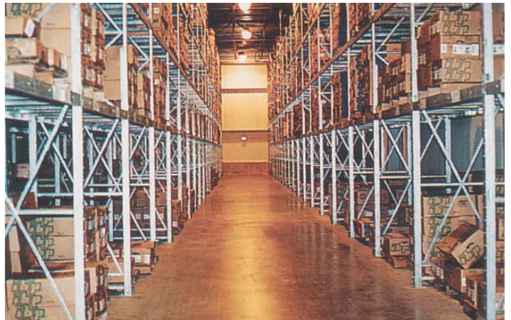
The new P&C facility utilizes narrow aisle configurations with stacking height to 32 feet clear in the freezer and 26 feet clear in the remaining ambient temperature areas, with racks provided by Frazier.
