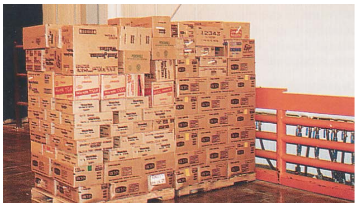
Using slotting techniques recommended by Kom International which emphasize factors such as case size and weight, selectors at P&C are able to build pallet loads of consistent case heights and weight distribution from heavy at the bottom to light at top.
