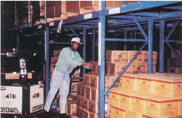
Picking bays were ergonomically designed to prevent unnecessary bending and twisting on the part of Bi-Lo's order selectors.
