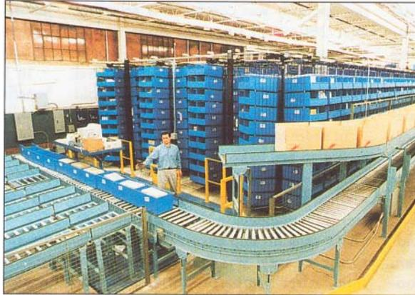
**Global's carousel system, consisting of four 10-foot-high strings, has taken over half the operation's volume.**
